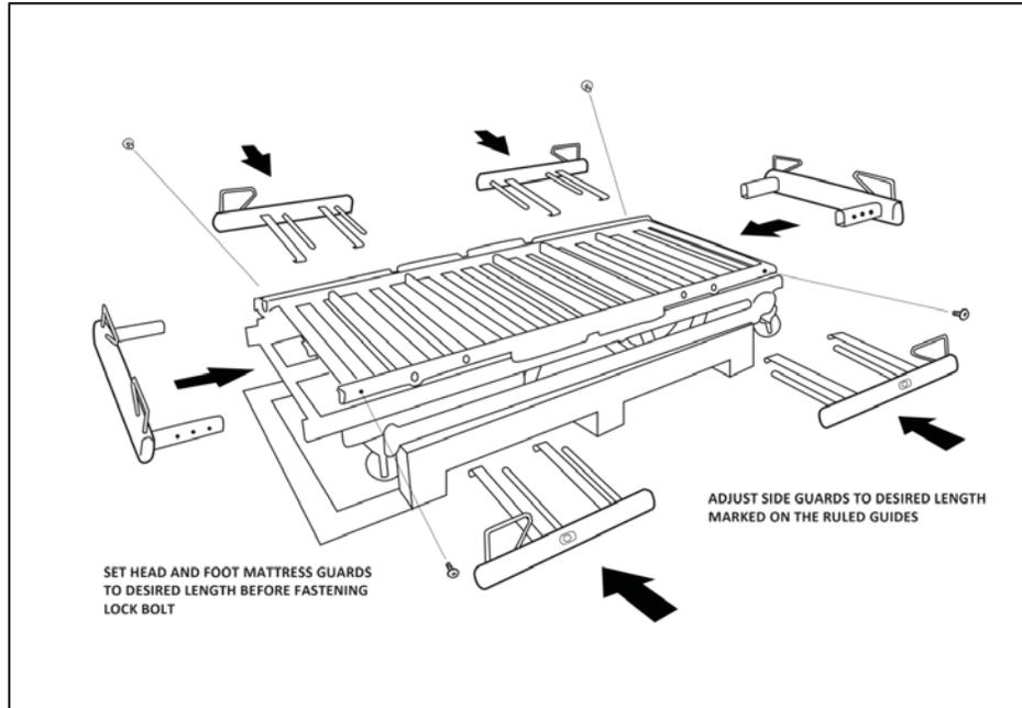
**Note:** Location of the head and foot mattress guards as well as the location of the side guards. Adjust all guards to the desired length and fasten head and foot guards using (4) of the small hex button head bolts and your 3/16 hex key wrench. **Correct guard placement shown below.**
